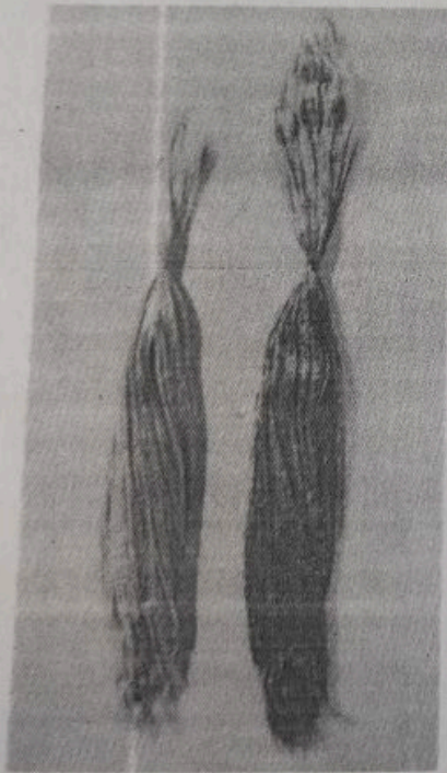
Figure 14-4 Emerging from the combing process, these long wisps of fiber have passed over a series of graduated metal pins in the combing machine and now resemble switches of human hair. The fiber at the left was retted in water; the fiber at the right was field retted. (Courtesy International Linen Association).
