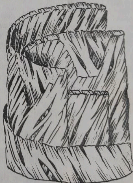
Figure 13-4 Diagram of inner layer of an enlarged cotton fiber shows how fibrils crisscross and double back. This structure contributes greatly to the strength of cotton. (Courtesy CIBA Review)
