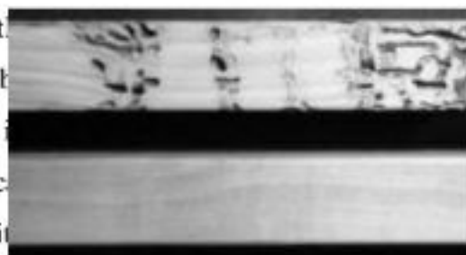
Figure 16. Non-treated and acetylated wood under biological attack
