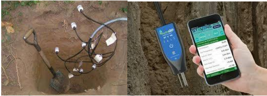
HYDRAPROBE soil moisture sensor for soil moisture, Ec and pH measurement
