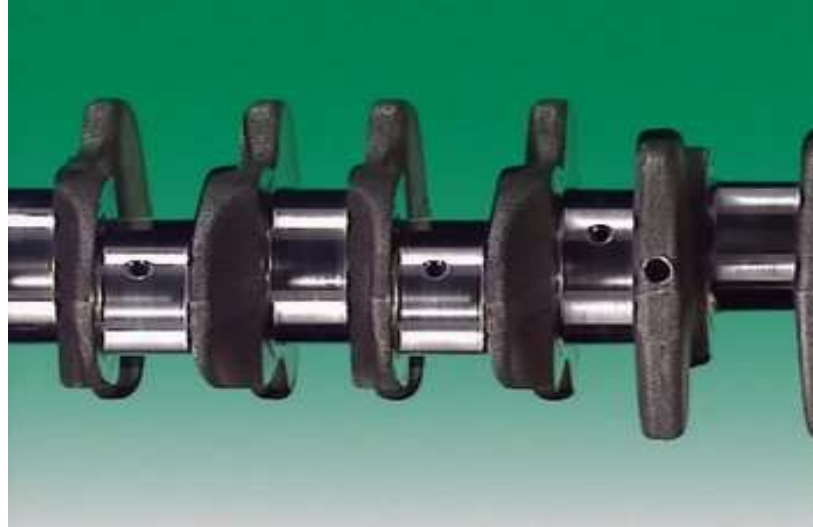
Oil spurt holes in crankshaft
