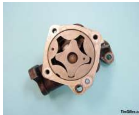
Star shaped rotor pump
